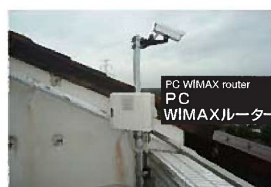
Portable camera installed on a building 可搬カメラの設置状況
